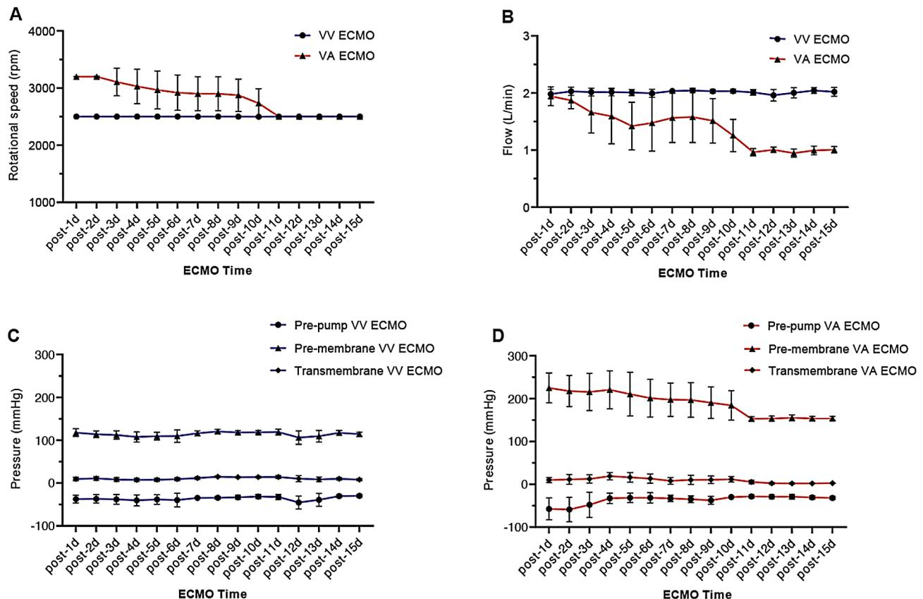
**Fig. 3** Specific Operating Parameters of the ECMO Device: **(A)** The rotational speed of the HR-ECMO system for all sheep; **(B)** The flow of the HR-ECMO system; The pre-pump pressure, pre-membrane pressure and transmembrane pressure of the HR-ECMO system for **(C)** VV ECMO group and **(D)** VA ECMO group; post-1d, the first day post the operation
