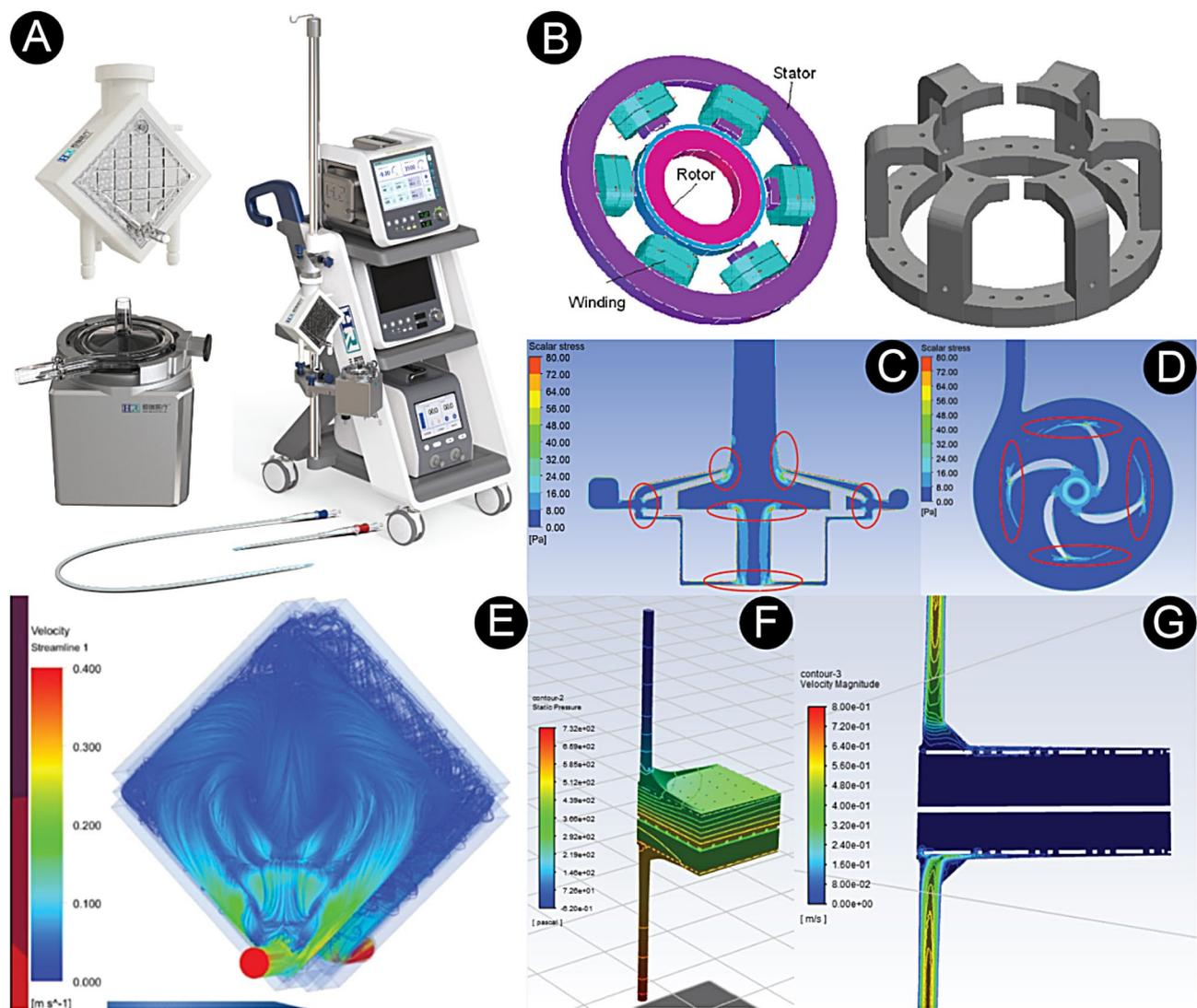
**Fig. 1** Hengrui Hongyuan Extracorporeal Cardiopulmonary Support System: (A) Appearance of the HR-ECMO system; (B) The basic internal structure of the pump; (C) The distribution of scalar stress in the central plane; (D) The distribution of scalar stress in the XY-plane; (E) The particle residence, (F) pressure distribution and (G) velocity distribution inside the membrane oxygenator
