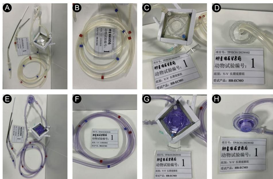
**Fig. 5** Observation of ECMO equipment after withdrawal and heparin coating staining: (A, B, C, D) Circuit tubing, hollow fiber membrane and pump head before staining; (E, F, G, H) Circuit tubing, hollow fiber membrane and pump head exhibited a fairly uniform bluish-purple coloration after staining with toluidine blue, indicating that the heparin coating was relatively intact
