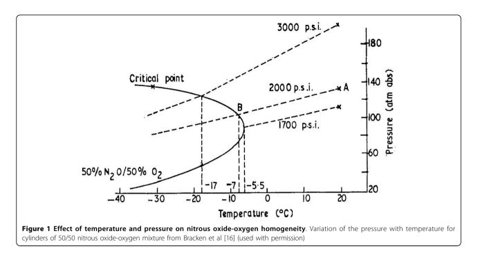
a cylinder filled to 138 bar (2,000 psig); at 207 bar (3,000 psig) the value decreases further to  $-17^{\circ}$ C.
